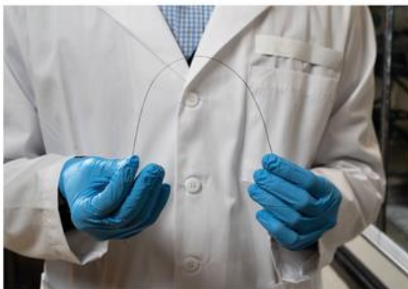
▶ The membranes for paraxylene separation will be fabricated in the form of hollow fibers. The thread-like fibers used to make these membranes will need to be produced by the hundred million for industrial use.
